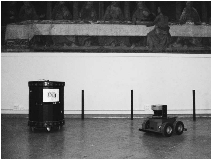
Fig. 7. Experimental setup: the mobile robots Nomad XR4000 (left) and Pioneer 3AT (right)
