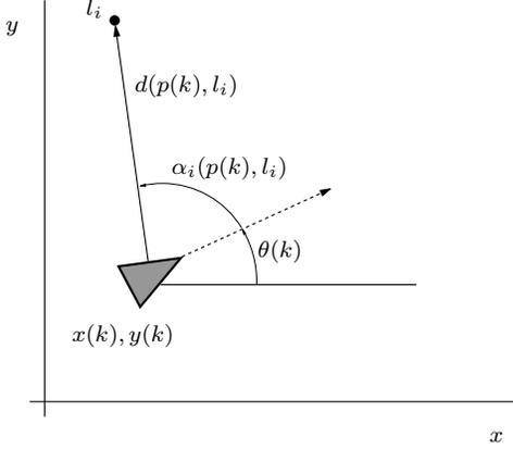
Fig. 1. Range and bearing measurement with respect to the  $i$ -th landmark.
