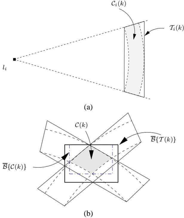
Fig. 2. (a) Trapezoidal approximation of a sector of corona. (b) Outer approximation of the exact feasible position set  $C(k)$  (dashed region) related to two landmarks.
