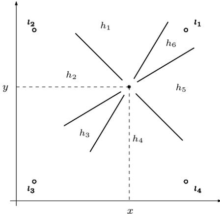
Fig. 3. Example of orientation partition: asterisk denotes the robot position  $z = [x, y]'$ , circles represent landmark positions, solid lines bound the angular subsets  $h_i$ .
