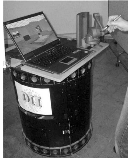
Fig. 1. MHI based on the holonomic Nomad mobile robot and a desktop PHANToM.
