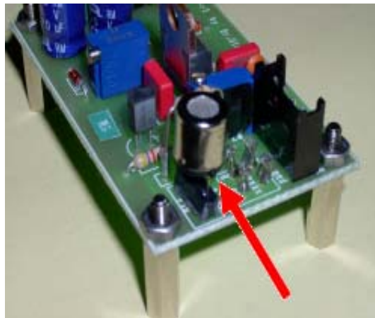
Figure 9: correct placement for FIS gas sensors.
